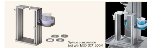
Syringe compression test with MED-SCT-500N
