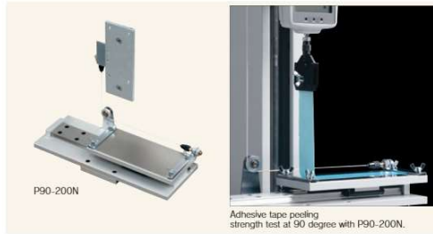
Adhesive tape peeling strength test at 90 degree with P90-200N.
