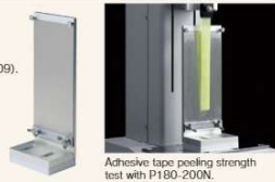
Adhesive tape peeling strength test with P180-200N.
