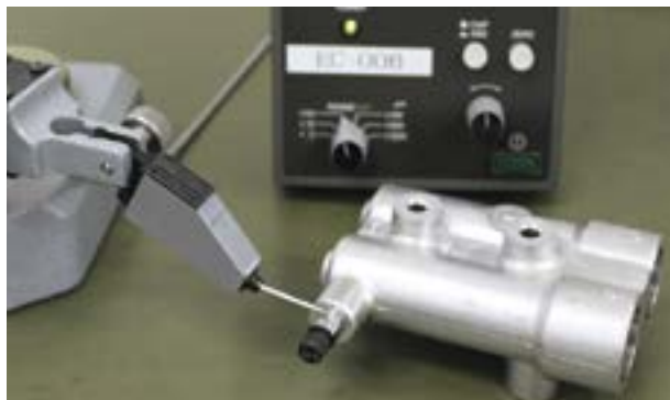
基準面からのねじ穴高さ測定(インジケータ測定) For measuring threaded hole height/length from the datum (using indicator)
